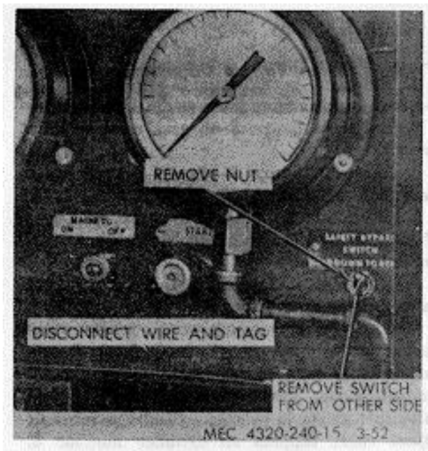
Figure 3-52. Safety bypass switch removal and installation.
